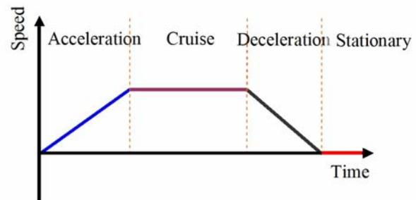
Fig. 1 Ideal speed profile for stop/start cycle
