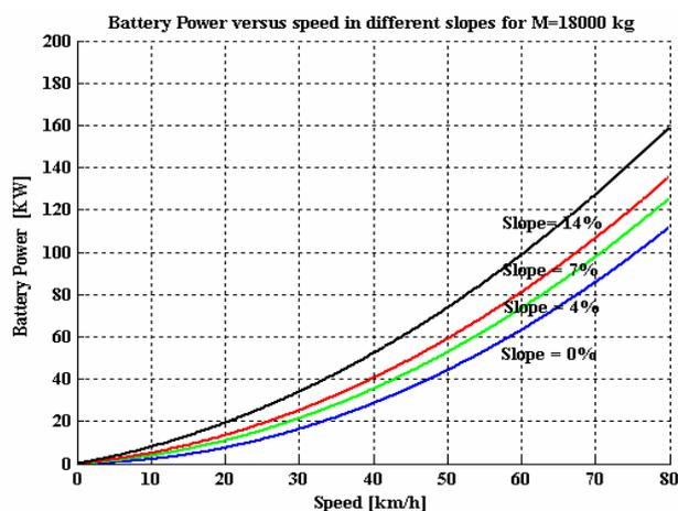
Fig. 6 Battery Power versus vehicle speed on the different slopes
