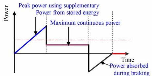
Fig. 2 Corresponding theoretical power demand by the propulsion
