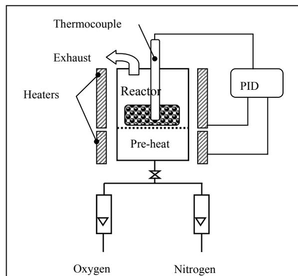
Fig. 1 Schematic Diagram of Fixed Bed Pyrolysis System
