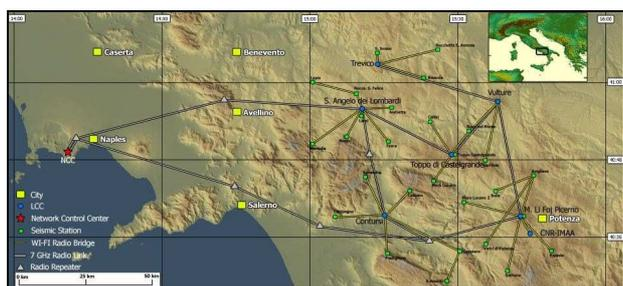
Fig. 3 Topology of communication system of Irpinia Seismic Network (ISNet) in southern Italy
