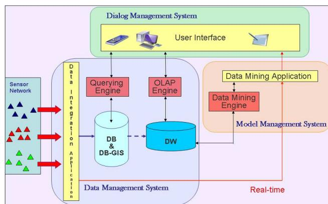
Fig. 15 Logical Architectural View of Seismic EW System
