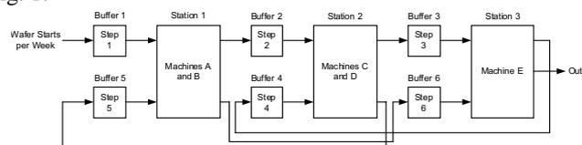
Fig. 1 The Intel five-machine six step Mini-Fab [19].
