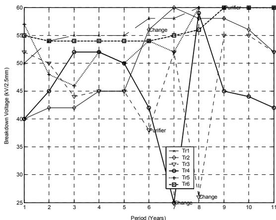
Fig. 1 Effect of service period on the breakdown voltage of the transformer oil
