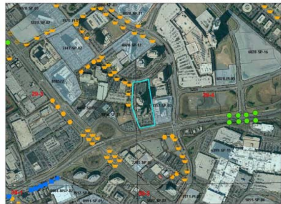
Fig. 1 Visual GIS display of a neighborhood with symbols and labels indicating the type of streetlights used.
