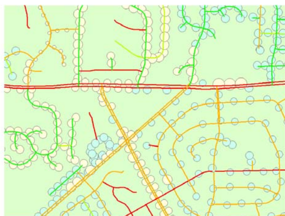
Fig. 3 Intersection between the effectively lit circle with the centerline of streets. Blue circles represent Mercury Vapor lamps. Two lines represent centerline of two way streets.
