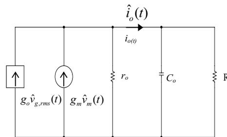
Fig. 8 Small signal ac frequency modeling of the boost pre-regulator with the proposed control method (where  $C_o$  = the output capacitor of the boost converter and  $R$  is the output resistor of the boost converter)
