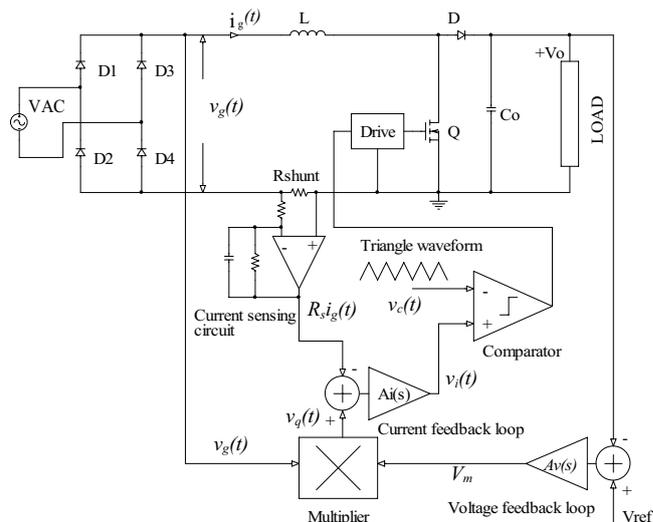
Fig. 1 Boost PFC converter with conventional controller
