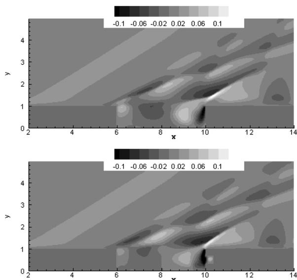
Fig. 7 Instantaneous contours of the stream normal flux of  $\rho v$  for the open cavity without the rear wall treatment (7a – upper) and with the rear wall treatment (7b – lower). The rest of the conditions are as in Fig. 4
