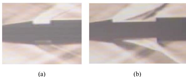
Fig. 3 Schlieren images for open-cavity of  $L/D=4$  (3a) and closed-cavity of  $L/D=12$  (3b) on the right
