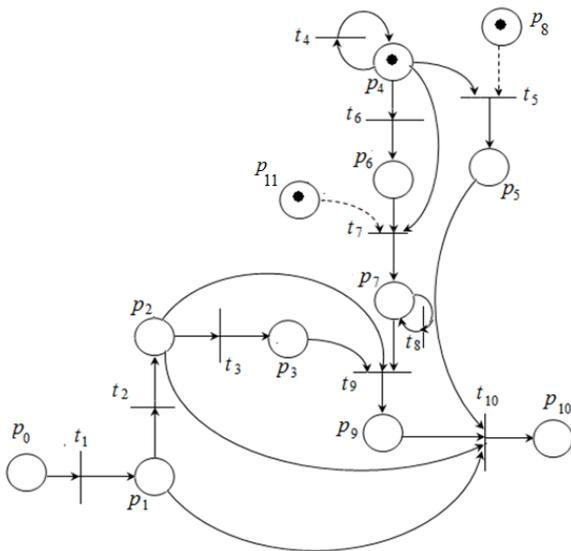
Fig. 2 Kalman Filter estimator Petri Net Model
