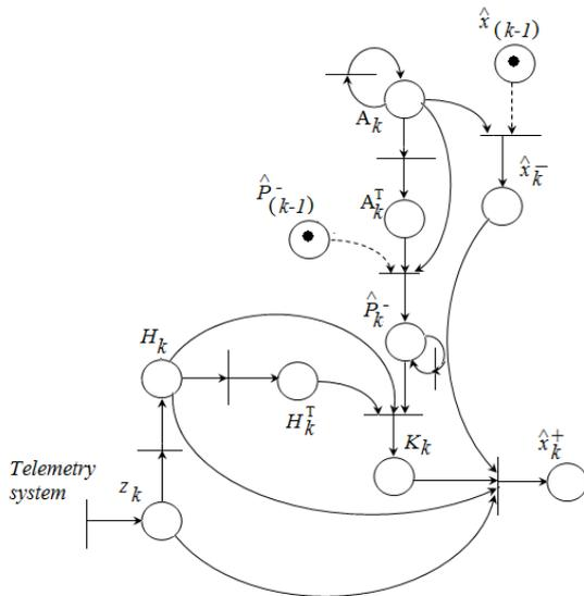
Fig. 1 Kalman Filter estimator Petri Net Algorithm
