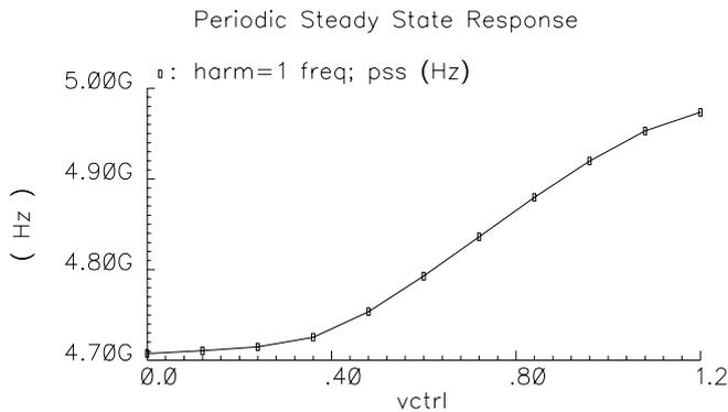
Fig. 8. VCO Oscillation Frequency vs.  $V_{CTRL}$ .
