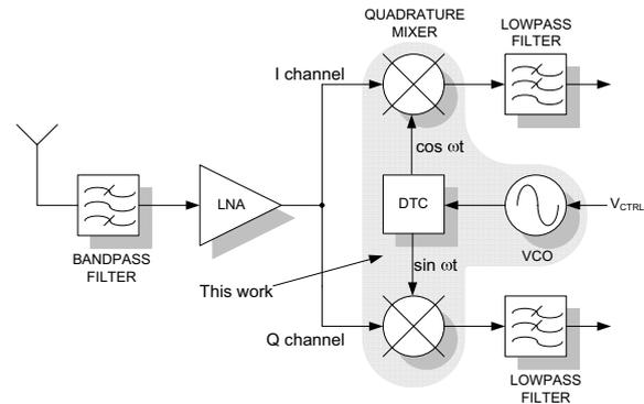
Fig. 1. Direct Down-conversion Front-End.
