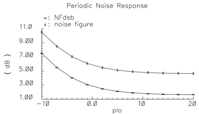
Fig. 4. Simulated Mixer Noise Figure at 1 KHz.
