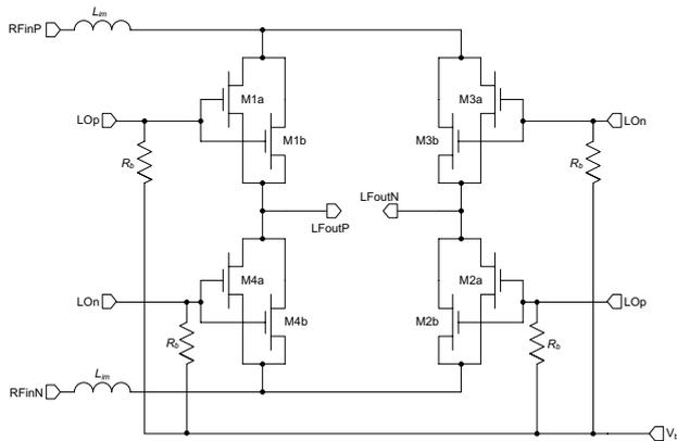
Fig. 2. The Passive Switch Mixer.
