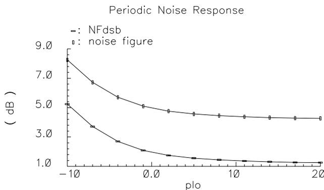
Fig. 3. Simulated Mixer Noise Figure at 10 MHz.
