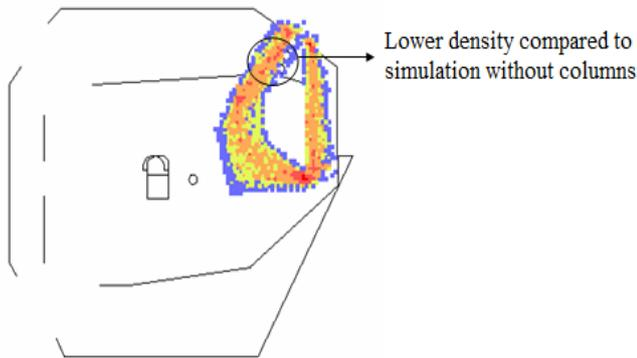
Fig.11 Simulation run for bottleneck area with columns.
