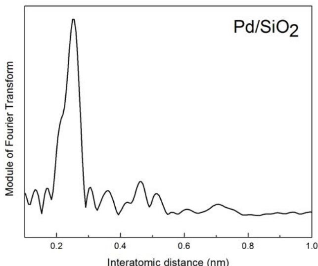
Fig. 4 The Fourier transforms of the EXAFS spectra for Pd supported on SiO<sub>2</sub>.
