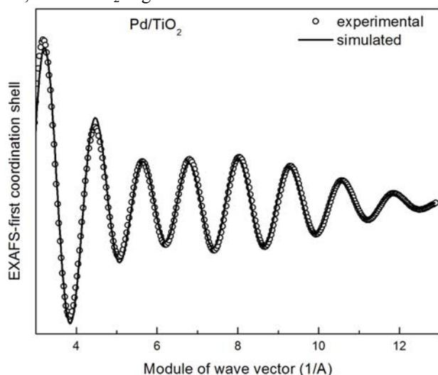
Fig. 5 The experimental and calculated EXAFS signals of the first coordination shell of Pd atoms for Pd supported on TiO<sub>2</sub>.
