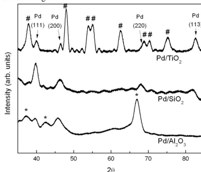
Fig. 1 XRD patterns of the investigated samples. The symbols indicate the XRD peaks associated to the metal oxides supports: #-TiO<sub>2</sub> (anatase) and \*- $\gamma$ -Al<sub>2</sub>O<sub>3</sub>
