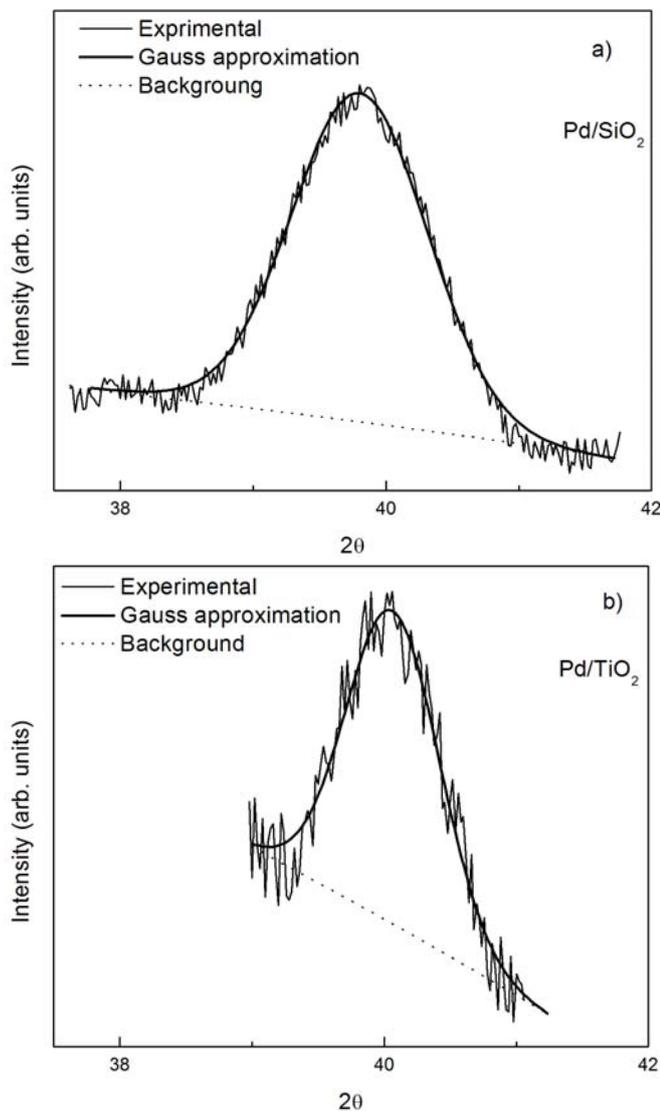
Fig. 2 Pd (111) XRLP of Pt/SiO<sub>2</sub> (a) and Pt/TiO<sub>2</sub> (b) approximated with an analytical Gauss function type
