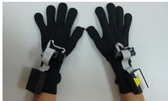
Fig. 1 Optical fiber gloves
