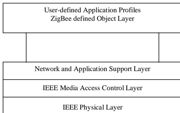
Fig. 3 IEEE 802.15.4 / ZigBee Stack Architecture
