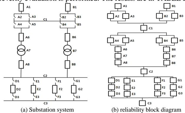
Fig. 2 Power substation system and reliability block diagram
