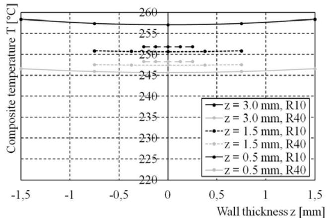
Fig. 16 Temperature distribution through composite sheets using *HS3*
