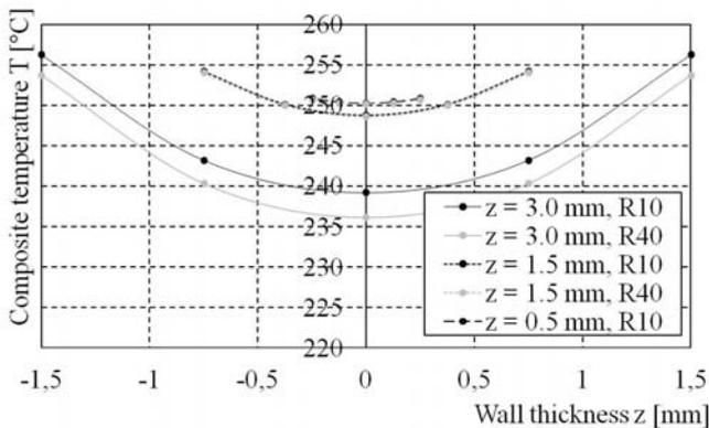
Fig. 14 Temperature distribution through composite sheets using *HS1*
