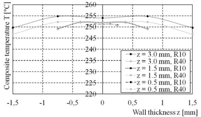
Fig. 15 Temperature distribution through composite sheets using *HS2*
