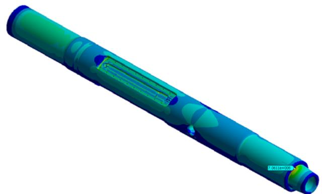
Fig. 4 von-Mises stress distribution for Case 3 loading
