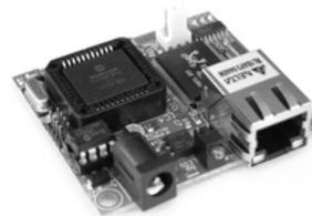
Fig. 1 Modtronix SBC45EC board
