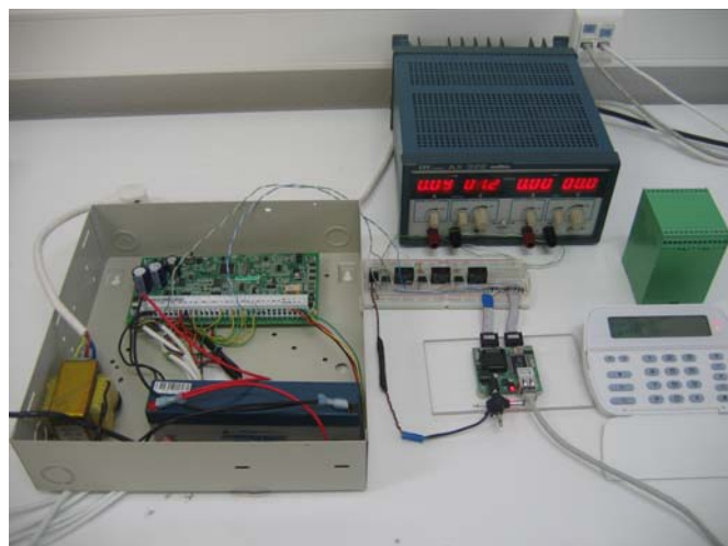
Fig. 6 Alarm system and external keypad connected to the working I/Os circuit and the micro web-server board
