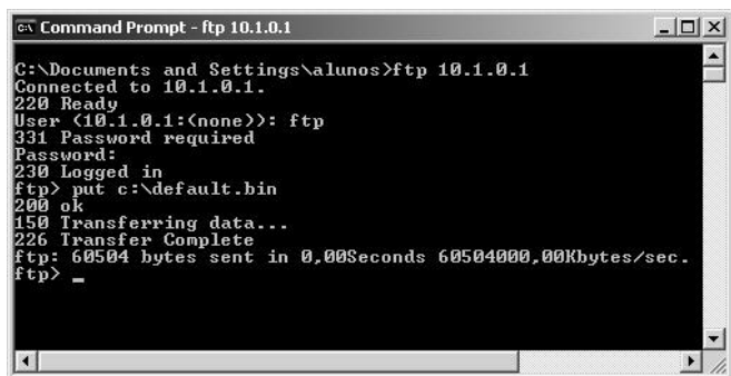
Fig. 8 FTP commands for programming the micro web-server with the default.bin file
