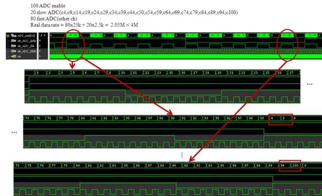
Fig. 8 The simulation result of IC1 (4M)
