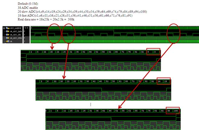
Fig. 7 The simulation result of IC1 (0.5M)
