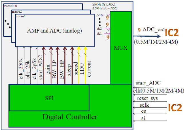
Fig. 2 Block diagram of IC1
