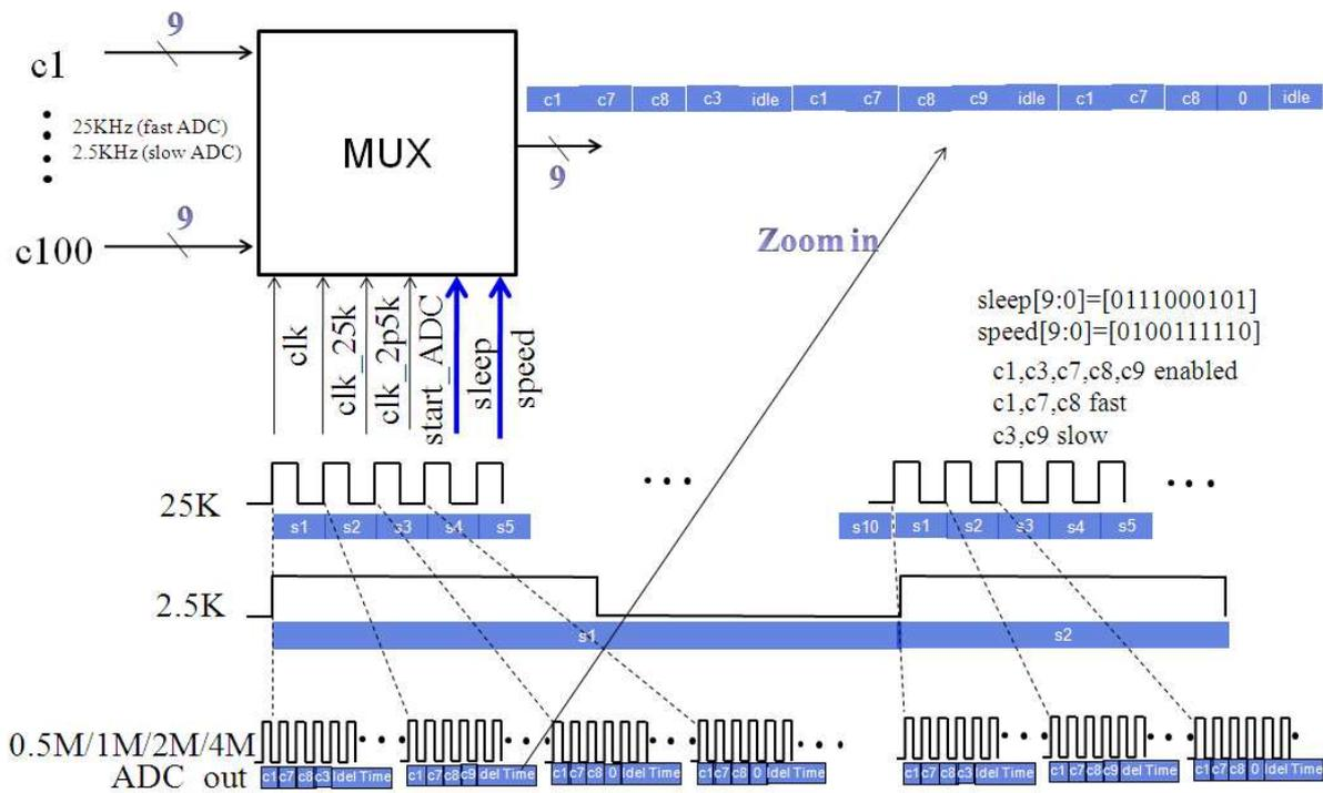
Fig. 3 The schematic diagram of the multiplex
