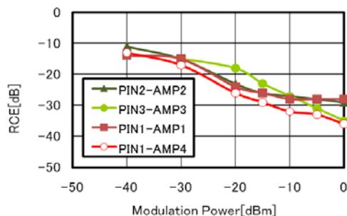
Fig.7 RCE measurement of four different O/E converters
