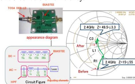
Fig.1 TOSA type E/O converter with Bias-Tee and adjusted input impedance on Smith Chart
