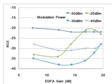
Fig.11 RCE measurements result with various EDFA gains.
