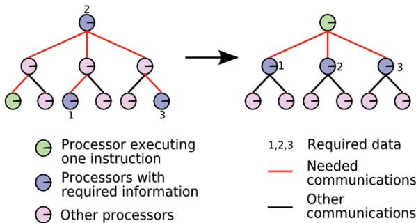
Fig. 4. Example of the reconfiguration of a HNoC applied to a distributed database. At least 3 nodes have changed its master/slave role, to adapt the HNoC network topology to the data distribution. This has been made in order to minimize the global delay for the execution of the query in the system.
