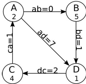
Fig. 2. Example of a System Graph  $G_S$ . The characteristics of the graph are: nodes  $P = \{A, B, C, D\}$ , links  $L = \{ca, ab, ad, bd, dc\}$ , processing weights  $\tau = \{2, 5, 4, 1\}$  communication latencies  $\delta = \{1, 0, 7, 1, 2\}$  and  $neig(A) = \{B, D\}$ ,  $path(C, D) = \{C, A, B, D\} \cup \{C, A, D\}$ , but  $path_{min}(C, D) = \{C, A, B, D\}$
