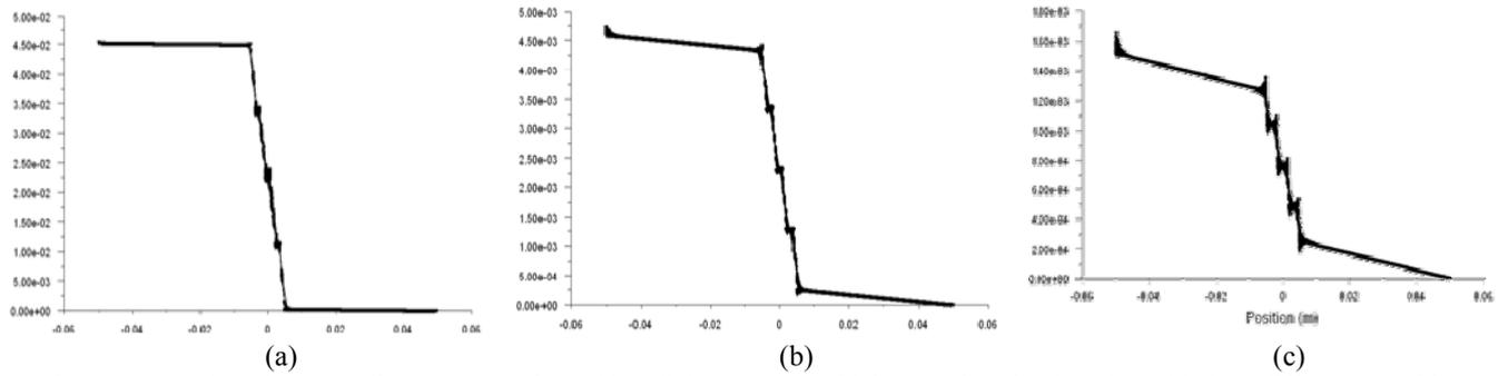
Fig. 8 Pressure drop through cellular structure for Cubic cellular structure with intersecting circular tubes with three different porosities (a)  $\epsilon = 0.17$ , (b)  $\epsilon = 0.51$  (c)  $\epsilon = 0.77$  (Pressure Vs. Position)
