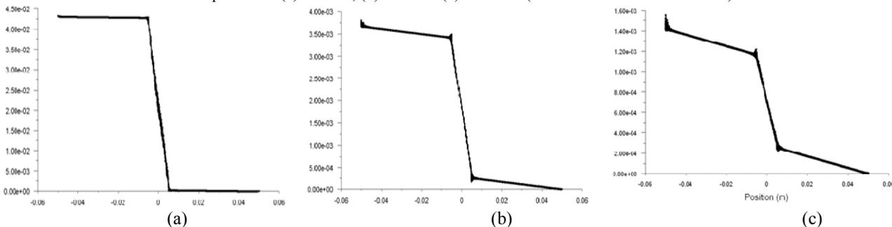
Fig. 6 Pressure drop through cellular structure for Cubic cellular structure with nine rectangular tube pores with three different porosities (a)  $\epsilon = 0.09$ , (b)  $\epsilon = 0.28$  (c)  $\epsilon = 0.71$ . (Pressure Vs. Position)
