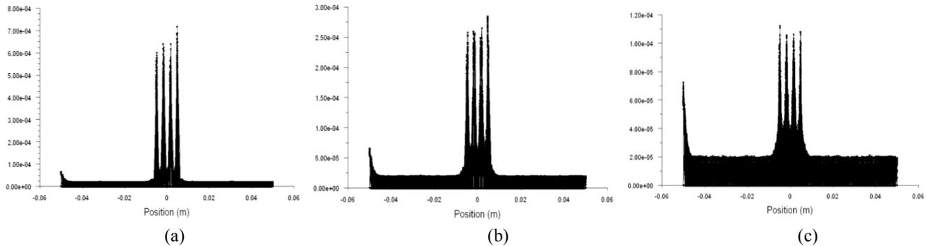
Fig. 13 Wall shear stress distribution through cellular structure for Cubic cellular structure with hollow sphere structure with three different porosities (a)  $\epsilon = 0.59$ , (b)  $\epsilon = 0.77$  (c)  $\epsilon = 0.89$  (wall shear stress Vs. Position)
