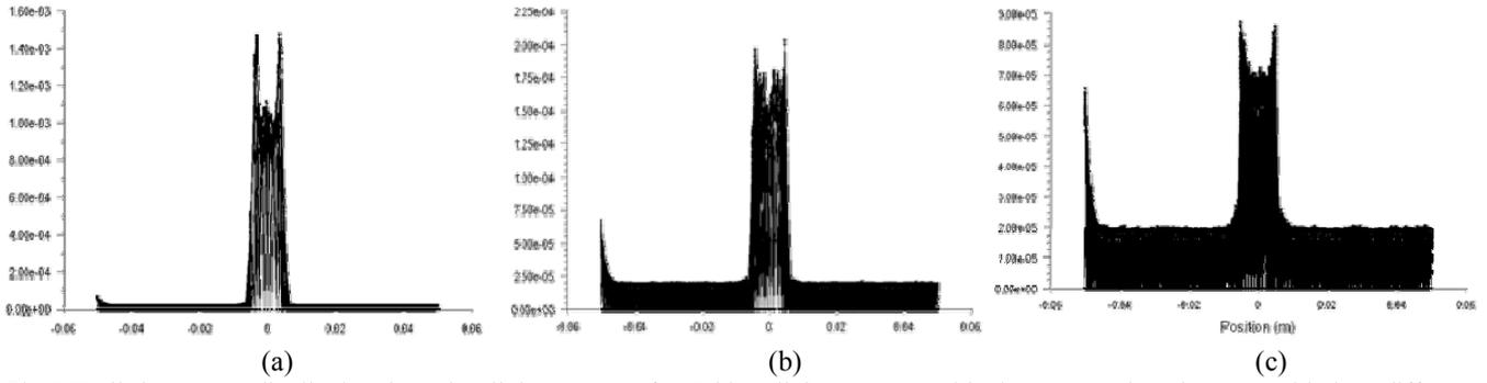
Fig. 7 Wall shear stress distribution through cellular structure for Cubic cellular structure with nine rectangular tube pores with three different porosities (a)  $\epsilon = 0.09$ , (b)  $\epsilon = 0.28$  (c)  $\epsilon = 0.71$  (Wall shear stress Vs. Position)
