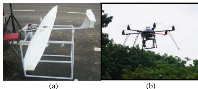
Fig. 1 (a) Fixed wing UAV; (b) Multi-rotor UAV
