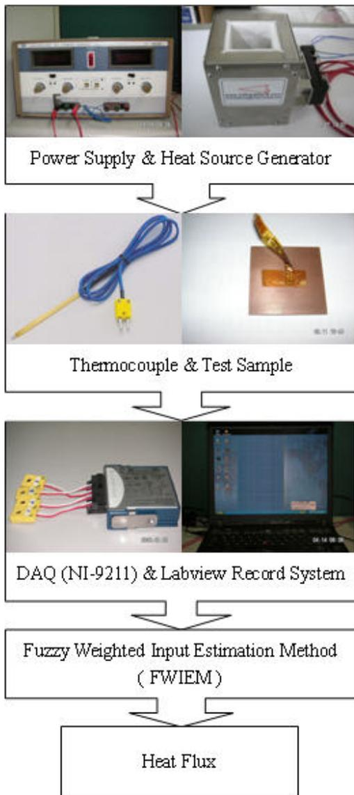
Fig. 1. The structure chart of the experiment.
