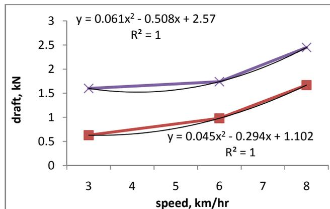
Fig. 2 Relationship between working speed and horizontal force (draft) in soil with 1.4 Mg m<sup>-3</sup>. (●) MDO, (■) DDO
