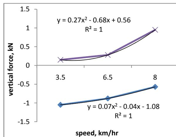
Fig. 3 Relationship between working speed and vertical force in soil with 1.4 Mg m<sup>-3</sup> (●) MDO, (■) DDO
