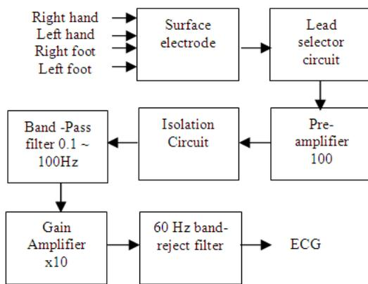
Fig. 2 Block Diagram of ECG Measurement Circuit
