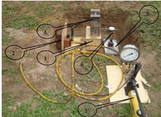
Fig. 1 The test set-up for determination of in-situ shear strength [1] hydraulic jack, 2) wooden plate, 3) metal box (approx.  $29 \times 15 \times 19 \text{ cm}^3$ ), 4) normal load, 5) metal plate, and 6) LVDT]
