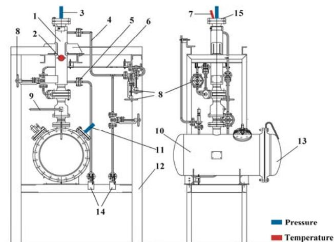
Fig. 1 Pre-treatment hydrolysis apparatus:
