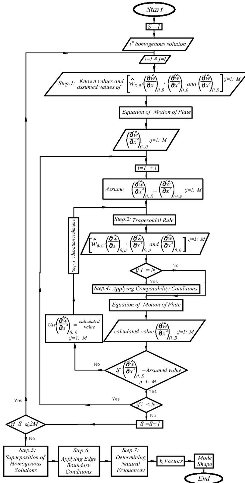
Fig. 2 Flow chart diagram of IVFD technique
