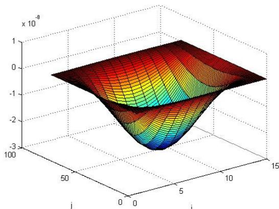
Fig. 3(a) 1<sup>st</sup>Mode shape of  $\lambda^2 = 26.1928$  and  $\alpha = 1.0$
