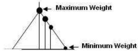
Fig. 1 Triangulation Weighting Function
