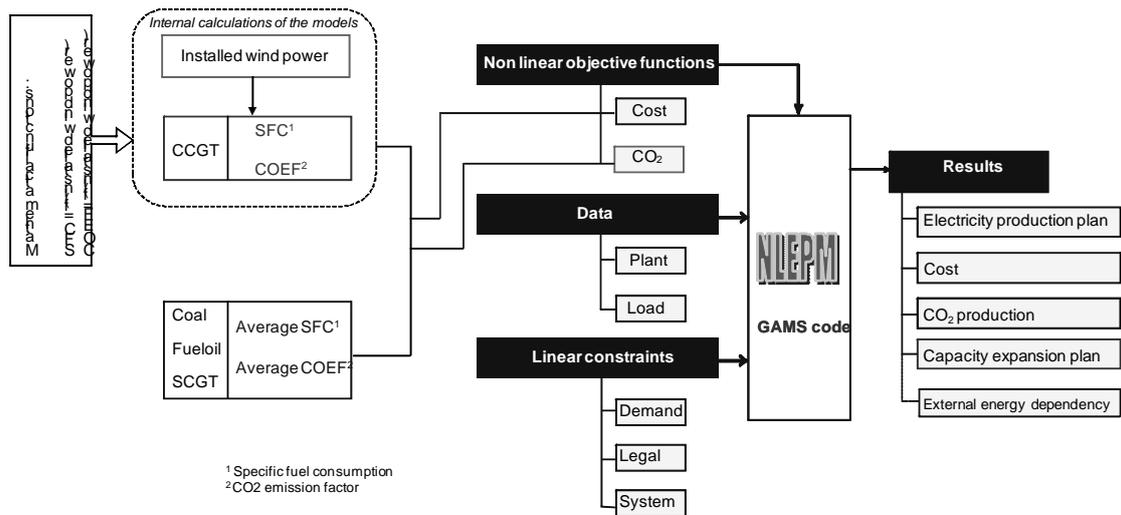
Fig. 2 Non linear electricity planning model (NLEPM)
