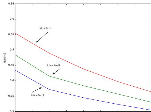
Fig. 5 Simulated relative 3<sup>rd</sup> harmonic current dependence on ac and dc-link inductance
