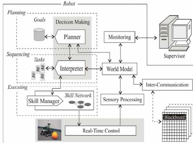
Fig. 5 Software Control Architecture for MRL Soccer Robots
