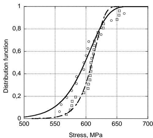
Fig. 3 Statistical distribution of static strength  $\sigma_0$  (circle symbols) and the calculated, according to (6), monotonic strength,  $\sigma_{0N}$  (square symbols), for T300/934 graphite/epoxy laminates. Broken and continuous lines represent the best fitting with a two parameters Weibull distribution for  $\sigma_0$  and  $\sigma_{0N}$ , respectively. Experimental data taken from reference [38]
