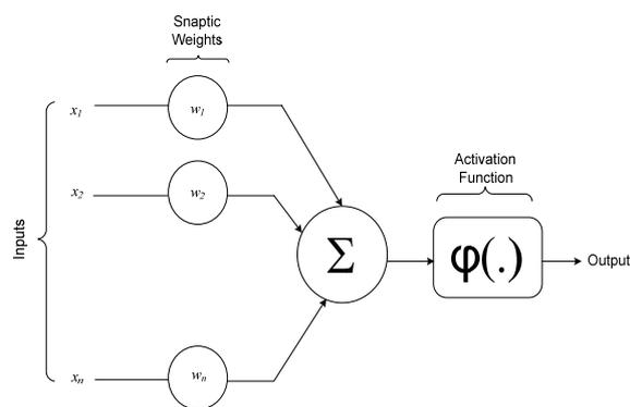
Fig. 1 Model of an artificial neural network
