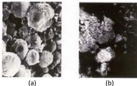
Fig. 3 Erosion debris from (a) SEDM (b) EDS
