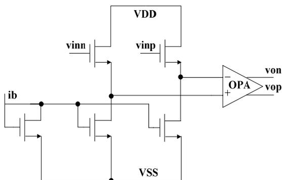
Fig. 2 The whole structure of the folded cascade OTA
