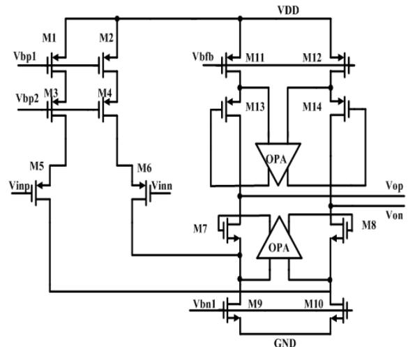
Fig. 1 The main form of the amplifier
