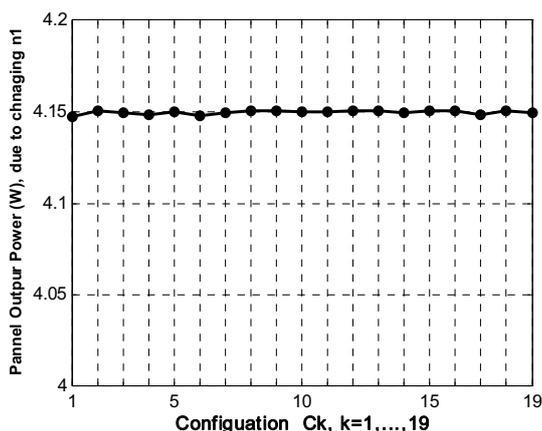
Fig. 10 Variation of panel output power for all layouts,  $U_1$  to  $U_{19}$  due to changing  $n_1$  from 0.9 to 1.0 for a temperature of  $27^\circ\text{C}$
