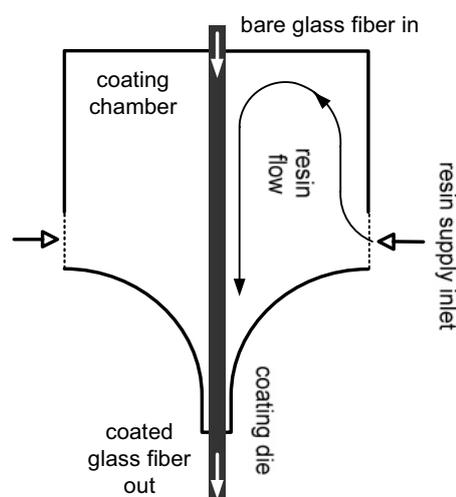
Fig. 1 Schematic of the optical fiber coating applicator
