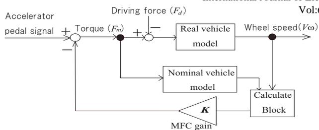
Fig. 6. Block diagram of model following control system
