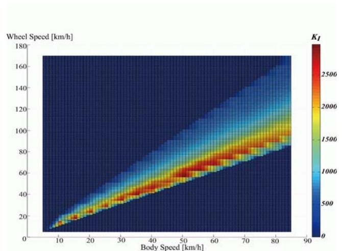
Fig. 5. Integral gain ( $K_I$ )
