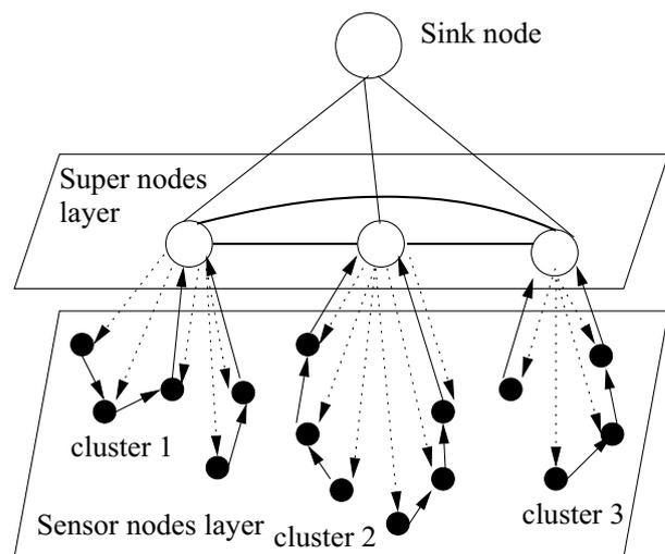
Fig. 1. Layered sensor network
