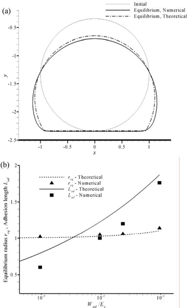
Fig. 5 Comparison between the numerical results and the results of the elastic model: (a) capsule shape at the equilibrium and (b) adhesion length and equilibrium radius of the capsule:  $W_{ad} = 4.11 \times 10^{-2} - 4.11 \mu\text{J}/\text{m}^2$ ,  $L_p = 0$ .
