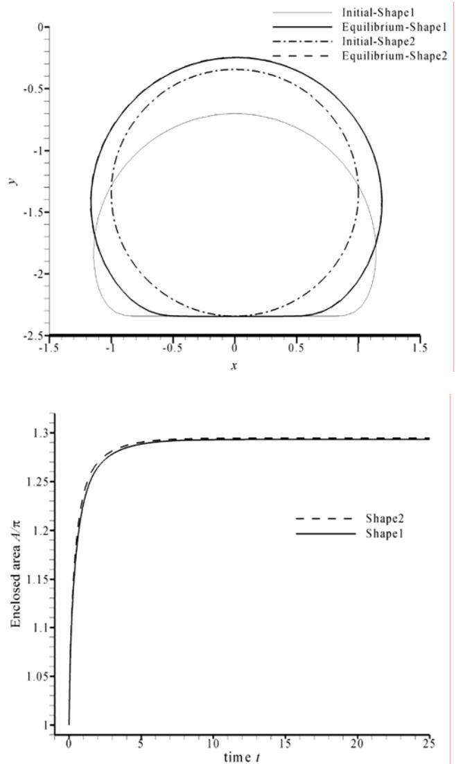
Fig. 9 Effect of the initial shape: (a) on the final equilibrium shape of the capsule and (b) on capsule swelling:  $W_{ad} = 4.11 \mu\text{J/m}^2$ ,  $L_p = 1 \times 10^{-8} \text{ m}^2\text{s/kg}$ ,  $\Delta c_0 = 10 \text{ mol/m}^3$ ,  $\gamma = 1.3586$ .
