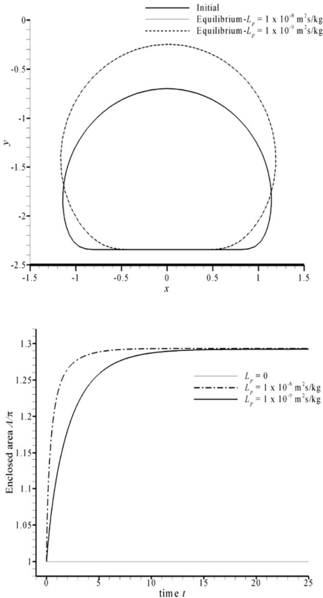
Fig. 8 Effect on the hydraulic conductivity: (a) on the final equilibrium shape of the capsule and (b) on capsule swelling:  $W_{ad} = 4.11 \mu\text{J/m}^2$ ,  $L_p = 1 \times 10^{-9}, 1 \times 10^{-8} \text{ m}^2\text{s/kg}$ ,  $\Delta c_0 = 10 \text{ mol/m}^3$ ,  $\gamma = 1.3586$ .
