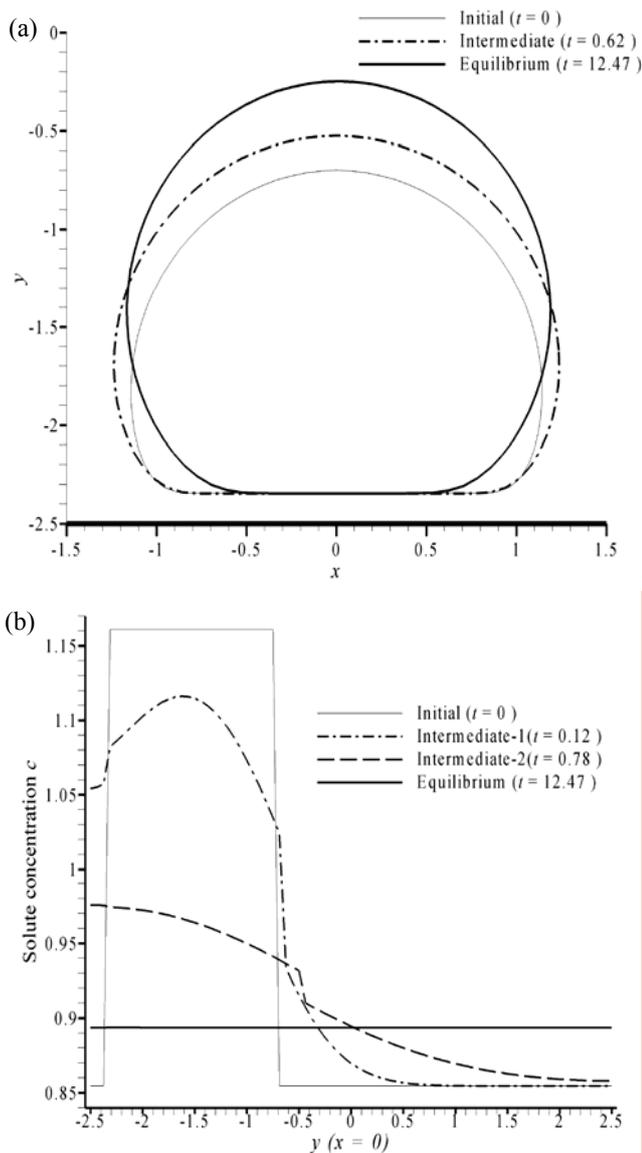
Fig. 6 Transient variation of capsule shape and solute concentration: (a) capsule shape under adhesion onto the planar substrate and (b) solute concentration filed on  $x = 0$  plane:  $W_{ad} = 4.11 \mu\text{J}/\text{m}^2$ ,  $L_p = 1 \times 10^{-8} \text{ m}^2 \cdot \text{s}/\text{kg}$ ,  $\Delta c_0 = 10 \text{ mol}/\text{m}^3$ ,  $\gamma = 1.3586$ .
