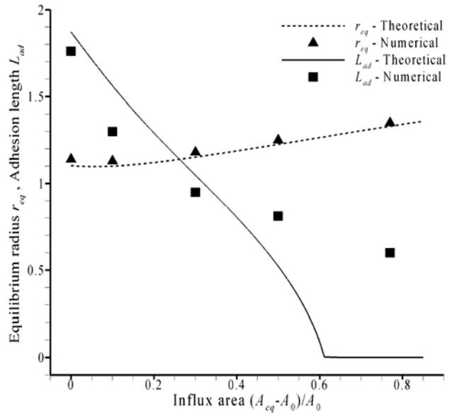
Fig. 7 Comparison between the numerical and theoretical solutions of the adhesion length and equilibrium radius of the capsule:  $W_{ad} = 4.11 \mu\text{J}/\text{m}^2$ ,  $L_p = 1 \times 10^{-8} \text{ m}^2 \cdot \text{s}/\text{kg}$ ,  $\Delta c_0 = 10 \text{ mol}/\text{m}^3$ ,  $\gamma = 1.116-2.000$ .
