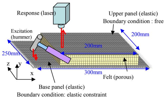
Fig. 3 Finite element model of test piece
