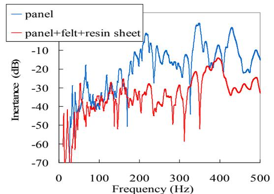
Fig. 2 Effect of porous media to reduce vibration of front floor (Excitation point: front cross member)
