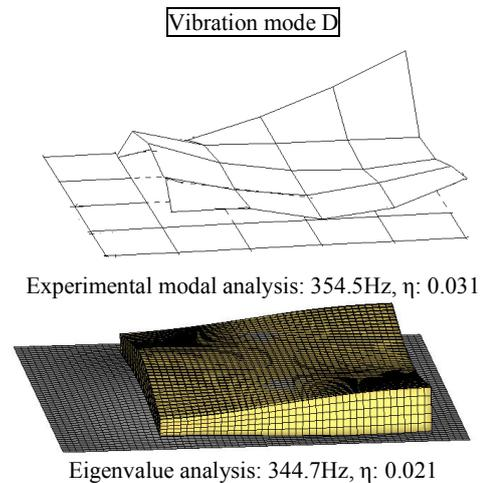
Fig. 9 Comparison of vibration mode D
