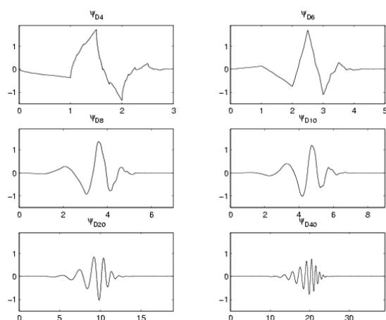
Fig. 2. Types of Daubechies Wavelet Transforms
