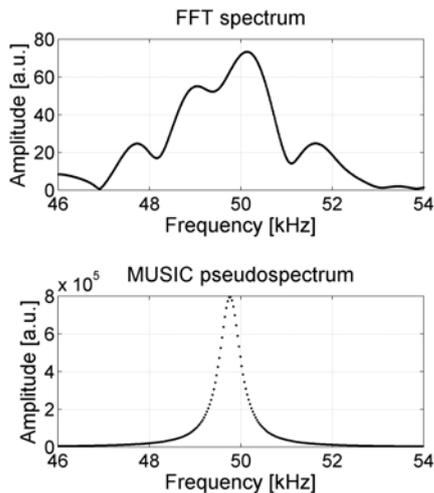
Fig. 5. Corresponding spectra to figure 4, calculated using FFT and MUSIC. The results are  $f = 50.13$  kHz for the FFT (predicted:  $f = 50.11$  kHz) and  $f = 49.77$  kHz for the MUSIC algorithm (prediction:  $f = 49.94$  kHz).
