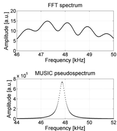
Fig. 7. Corresponding spectra to figure 6, calculated using FFT and MUSIC. The results are  $f = 47.27$  kHz for the FFT and  $f = 49.76$  kHz for the MUSIC algorithm (prediction for both methods:  $f = 48.00$  kHz).
