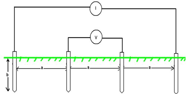
Fig. 2 Wenner Method for Soil Resistivity Test
