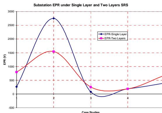
Fig. 11 Computed EPR under different soil Structure
