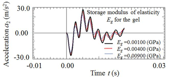
Fig. 14 Effects of elasticity  $E_g$  of the gel on dynamic errors of the force transducer
