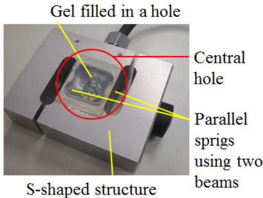
Fig. 2 Photo of the S-shaped force transducer [3]
