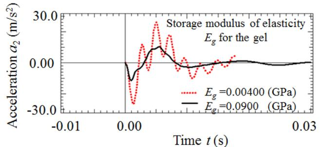
Fig. 11 Effects of elasticity  $E_g$  of the gel on dynamic errors of the force transducer
