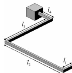
Fig. 2 The meandering legs used for anchoring
