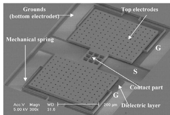
Fig. 1 The structure of the crab leg membrane
