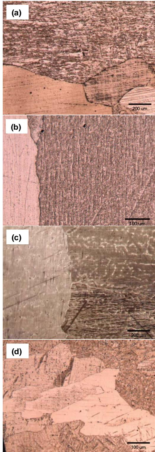
Fig. 3 As-cast microstructures of ingots of (a) pure Mg, (b) Mg-0.1Y, (c) Mg-1Zn-0.5Y, and (d) Mg-0.1Ce alloys
