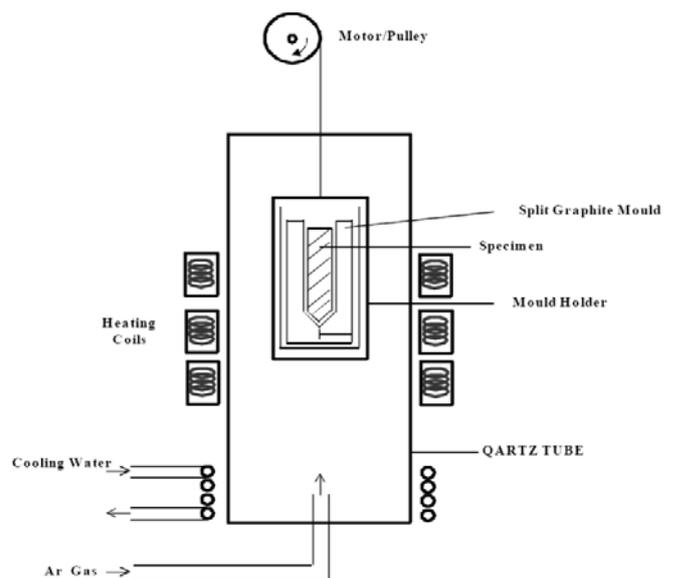
Fig. 1 Schematic illustration of the apparatus for single crystal growth
