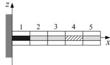
Fig. 4 Smart beam (actuator at 1<sup>st</sup> position, sensor at 4<sup>th</sup> position)
