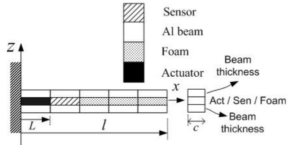
Fig. 2 Smart beam (actuator at 1<sup>st</sup> position, sensor at 2<sup>nd</sup> position)
