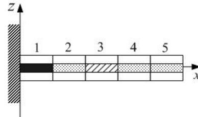
Fig. 3 Smart beam (actuator at 1<sup>st</sup> position, sensor at 3<sup>rd</sup> position)
