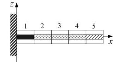
Fig. 5 Smart beam (actuator at 1<sup>st</sup> position, sensor at 5<sup>th</sup> position)
